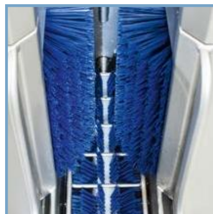
Walzenbürsten aus Nylon Roller brushes, made from nylon
